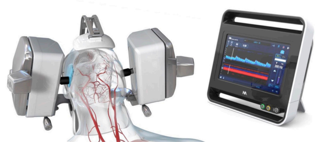
Fig. 6. The robotically assisted transcranial Doppler system used in this study (Neural Analytics Lucid Robotic System. Credit: Neural Analytics).
